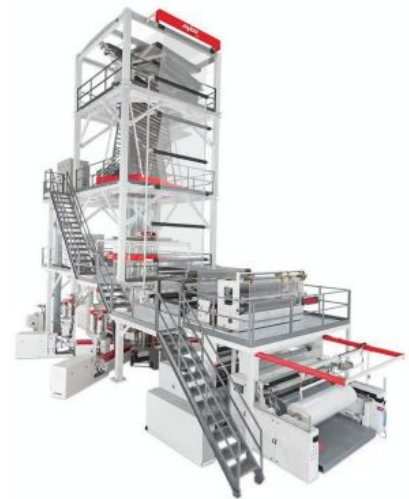
Rajoo's 5-layer blown film line
