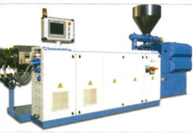
Rajoo and Bausano, Italy collaboration has given rise to India's first WPC (Wood Plastics Composite) Extrusion Machine. Construction, flooring, furniture and decking companies would significantly benefit as these machines come with a range of capacities (200 kg/hr to 1200 kg/hr) to manufacture profiles and boards that would use upto 80% of wood powder, a first ever in the industry
