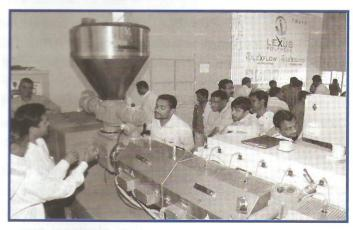
Twin Screw PVC Pipe Plant enthralled the audience when it was being operated at a capacity of 1000 kg/hr, never before seen in India. The pipe OD was 400mm and wall thickness of 16.2mm. This high output plant will now be shipped to Africa.
