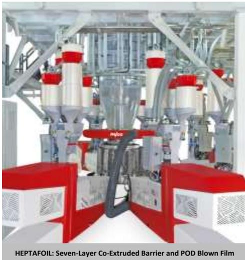
HEPTAFOIL: Seven-Layer Co-Extruded Barrier and POD Blown Film
