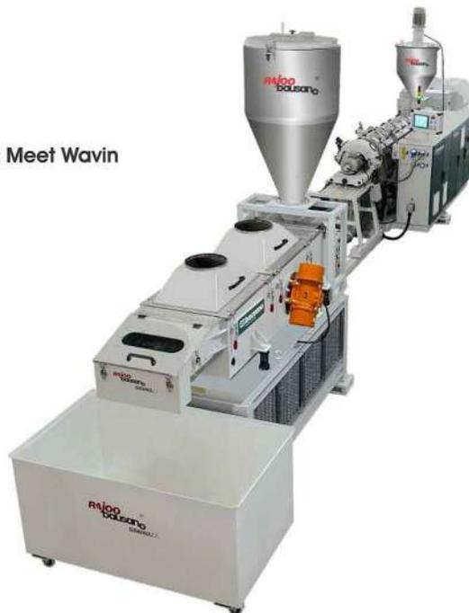
Wavin group opted for the Rajoo-BausanoGranulex (compounding + pelletising) system for its uPVC and cPVC fittings- a pioneering solution from Rajoo-Bausano which delivered a staggering output on 600 kg / hour; that too, at minimal energy consumption.
