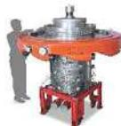
Developed CSD (Cylindrical Spiral Die) die head with rheologically optimized melt flow path for blown film line
