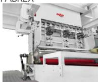
Developed Asia's first ever 65mm sheetline extruder for 180kg/hr output
