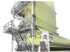
Introduced the first indigenously designed wide width blown film line for a lay-flat width of 3000 mm MULTIFOIL
