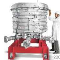
2005 Developed Asia's first three layer wide width blown film line incorporating die dia 1200 mm and 4000 mm LFW. The maximum output is 1200 kg/hr.
