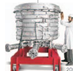
Developed Asia's first three layer wide width blown film line incorporating die dia 1200 mm and 4000 mm LFW. The maximum output is 1200 kg/hr.
