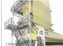
Introduced the first indigenously designed wide width blown film line for a lay-flat width of 3000 mm
