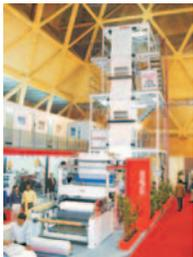
Launched Asia's highest output 3 layer blown film line with stack die (UCD) during Plastindia
