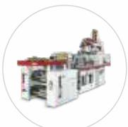
Developed and supplied first sheet line for physically foamed PE sheets using carbon dioxide as blowing agent
