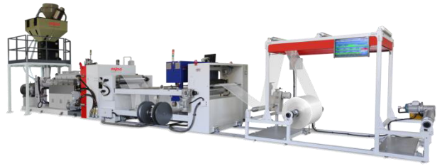
LAMINA ® - Mono & multilayer sheet lines for PP/EVA/PS
