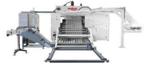
DISPOTILT - Tilting Mould Thermoforming Machine
