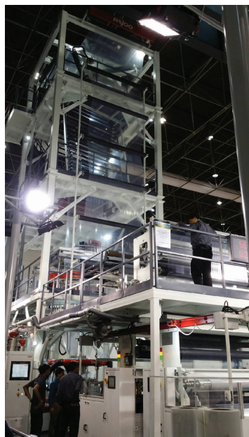
Rajoo's five-layer Pentafoil line shown at K2016 last year
