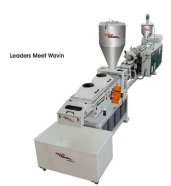
Wavin group opted for the Rajoo-BausanoGranulex (compounding + pelletising) system for its uPVC and cPVC fittings- a pioneering solution from Rajoo-Bausano which delivered a staggering output on 600 kg / hour; that too, at minimal energy consumption.
