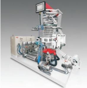
Source: world's smallest Three Layer Blown Film Lab Line-Labex.
