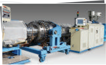
FLOWEX - Twin screw uPVC & CPVC pipe plant
